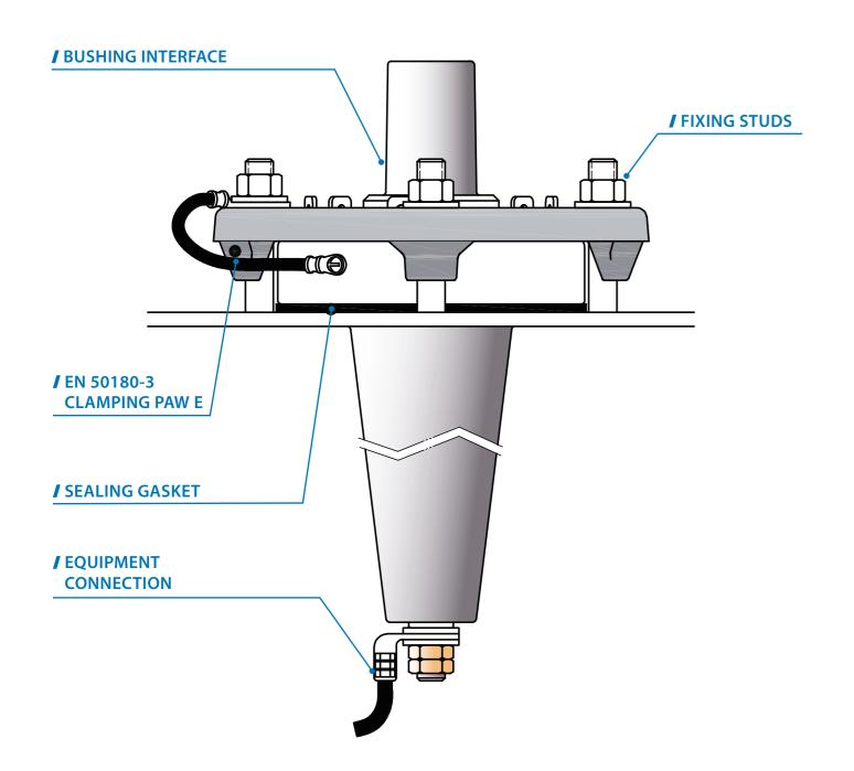
Fixings For Interface A1 Equipment Bushings EN 50180-3 & DIN 42 538
