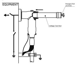
Clean and grease the test rod and front T-body interfaces. Insert the test rod into the front T-body and tighten the test rod at Hexagon Nut of stud to 20-25 Nm by Hex Wrench.
