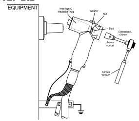
Tighten the stud to Interface C plug. Clean and grease the Interface C plug and front T-body interfaces. Insert the Interface C plug into the front T-body and put washer and nut on the stud. Tighten the nut to 50-55 Nm, using a torque wrench and a 24 mm socket.
