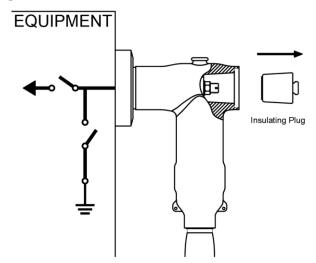
Unscrew and remove Insulating Plug. Make sure no contamination of T-body and Plug interface.
