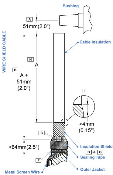
K PVC Tape 95mm(3.74") Sealing Tape 85mm(3.35") >5mm (0.2")
