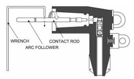
Rotate the elbow until the contact rod and arc follower align with the threaded hole of the connector. Thread the contact rod by hand to avoid cross-threading. Then, using the supplied wrench, tighten the rod until the wrench permanently deforms — this ensures proper torque.
