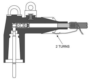
Use one or more neutral wires to connect the concentric neutral to the elbow's grounding tab near the cable entry. Ensure a tight, secure connection to guarantee effective grounding of the elbow shield.
