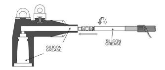
Apply a thin, even layer of silicone grease over the prepared insulation. Slide the elbow onto the cable using a steady twisting motion. Once seated, the elbow should align properly with the connector.
