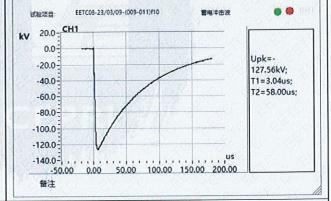
The 1st negative impulses waveform
