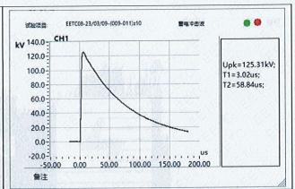
The 1st positive impulses waveform
