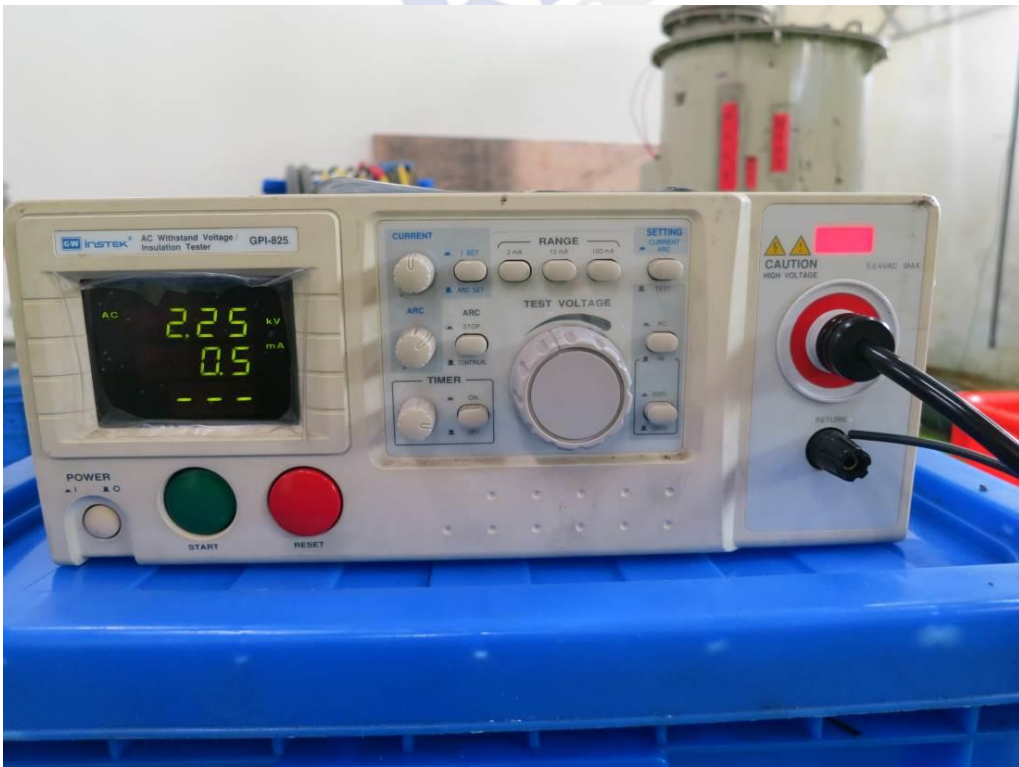
Voltage testing of the 2.2 kV 60Hz / 1min in water -III
