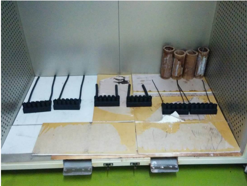
Oven conditioned at 113 \pm 5^{\circ}\text{C} -I
