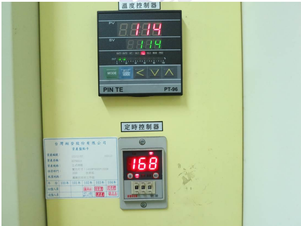
Oven conditioned at 113 \pm 5^{\circ}\text{C} -II
