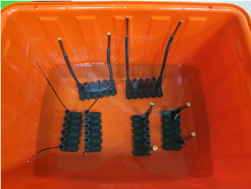
Sample in tap water at 25 \pm 5^{\circ}\text{C} for 4 h
