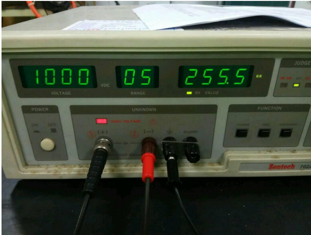
Insulation resistance measurement -II
