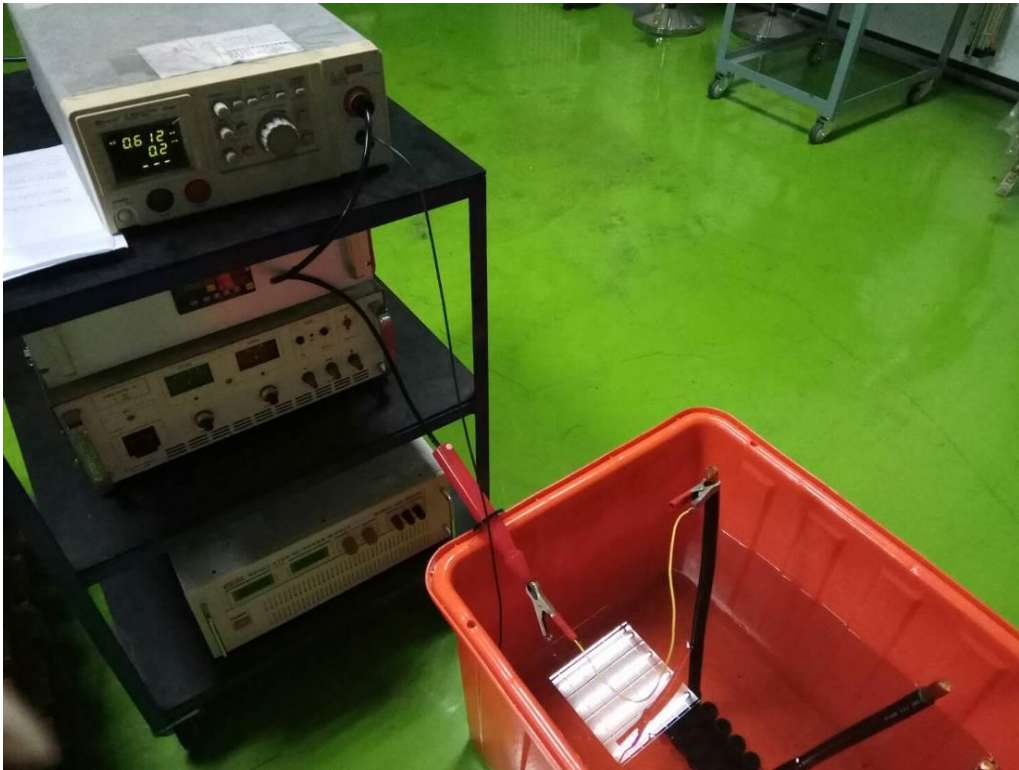
Leakage current test -I
