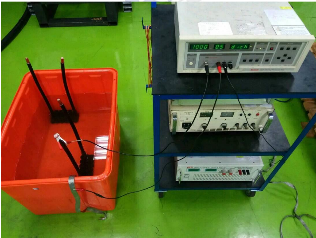
Insulation resistance measurement -I
