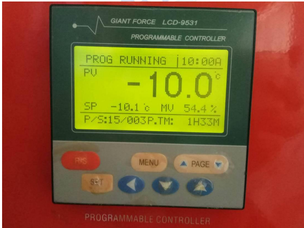
Cold conditioned at minus 10 \pm 2^{\circ}\text{C} -II
