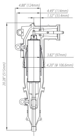
Fig 2: Dimension Info When CPS Fuse or Chardon Fuse Installed.
