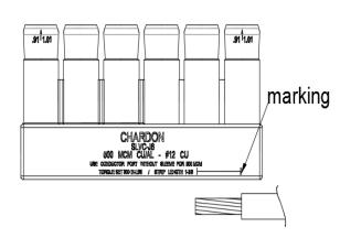
Measure the strip length. Place the cable alongside the markings on the body, strip the cable.
