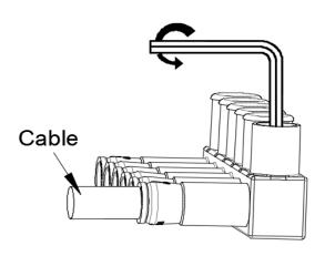
Insert torque tool and rotate it.(120in-lb for #12 to #4, 240in-lb for #2 to 500kcmil)
