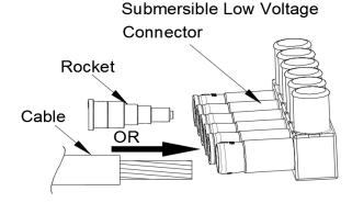
Insert the cable into the tower (500 kcmil) or the rocket (#12 to 350) until the end of the conductor reach the end of the window.
