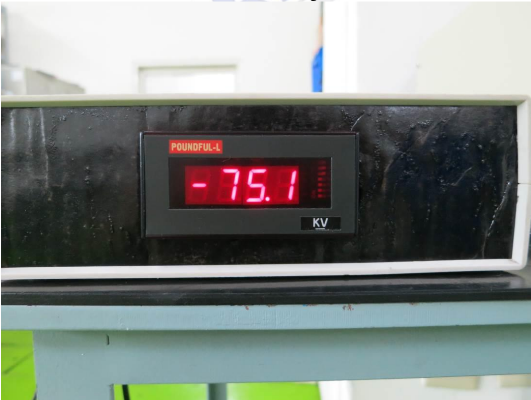
DC Withstand Voltage Test in Progress
