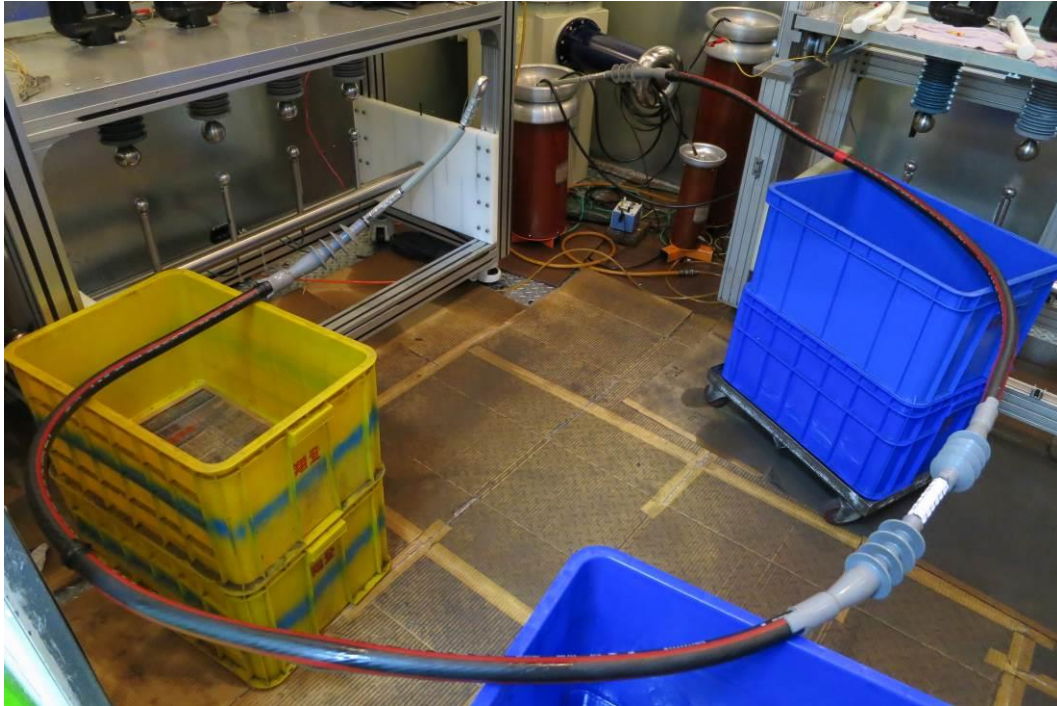
Partial Discharge Test
