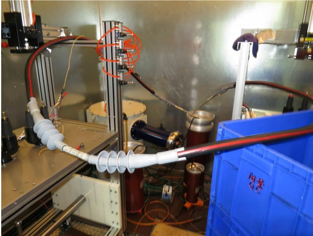
Partial Discharge Test
