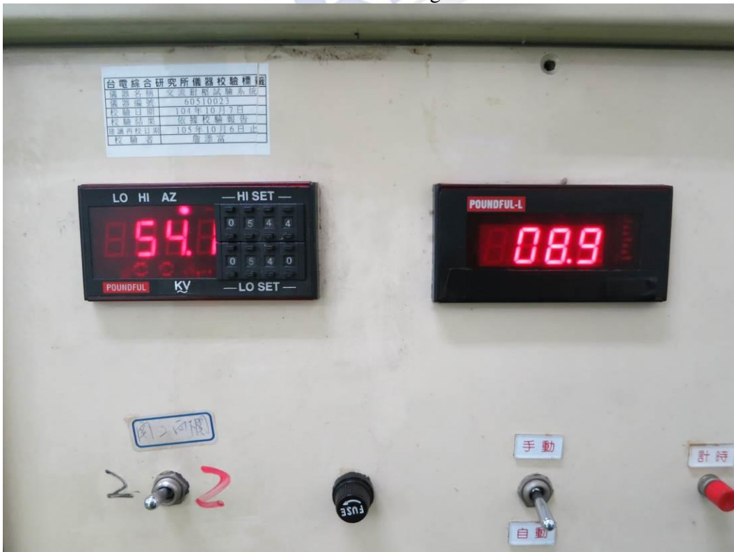
AC Withstand Voltage Testing in Progress
