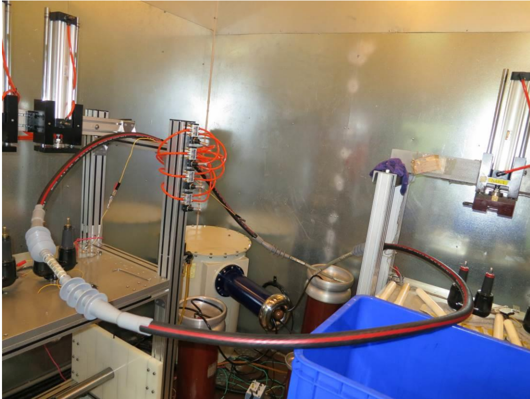
Partial Discharge Test
