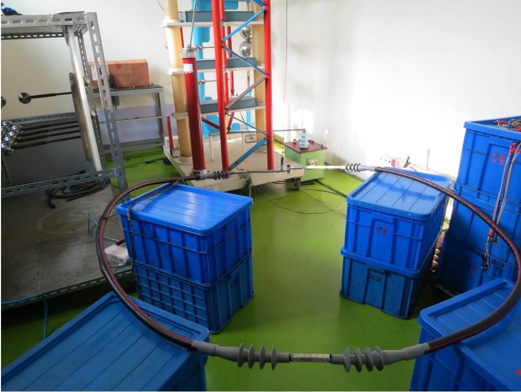
Impulse Withstand Test
