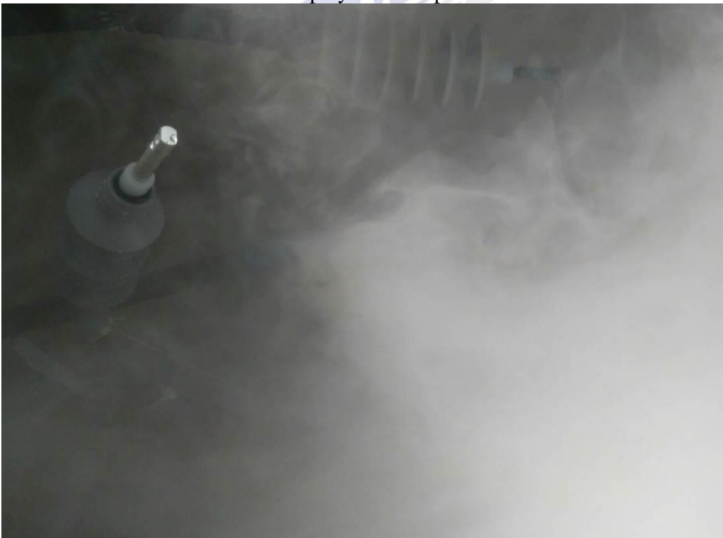
Salt Spray Test in Progress
