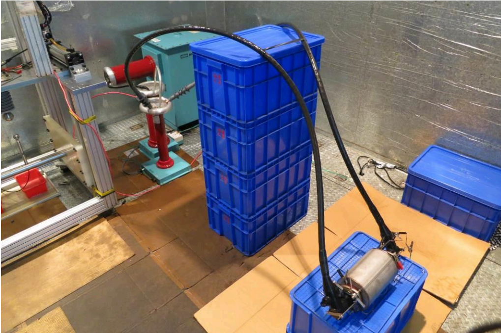
Testing Setup of AC Voltage Dry Test
