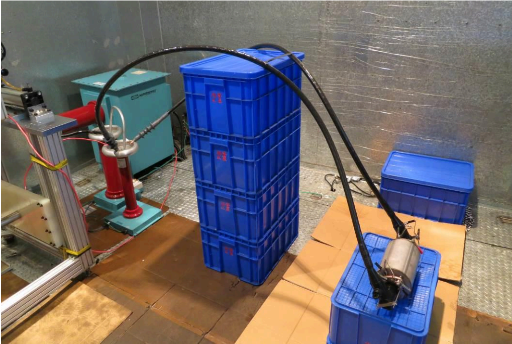
Testing Setup of Partial Discharge Testing
