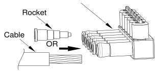
Insert the cable into the tower (250 to 350 kcmil) or the rocket (#12 to 4/0) until the end of the conductor reach the end of the window.
