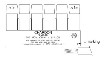
Measure the strip length. Place the cable alongside the markings on the body, strip the cable.
