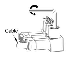
Insert torque tool and rotate it.(120in-lb for #12 to #4, 240in-lb for #2 to 350kcmil)
