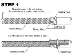
Remove cable jacket (if jacketed cable is used) to expose neutral wires. Provide Part No:401104P000 sufficient length of neutral wires for grounding after installation.
