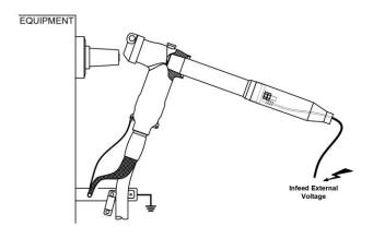
Connect test cable of external voltage to the stud of test rod. Push the insulating cover to the end of test rod. Infeed external voltage.
