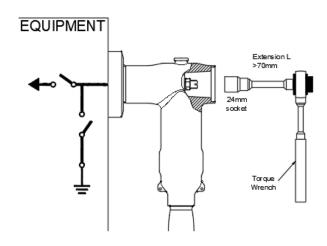
Check the nut at correct position and tighten to 50-55 Nm, using a torque wrench and a 24 mm socket.
