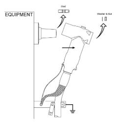
Unscrew and remove the Nut and Washer. Push the Front T-body out of equipment bushing and unscrew stud of equipment bushing.
