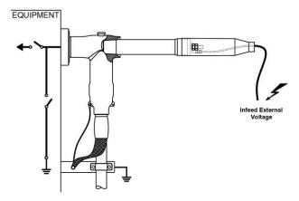
Connect test cable of external voltage to the stud of test rod. Push the insulating cover to the end of test rod. Infeed external voltage.
