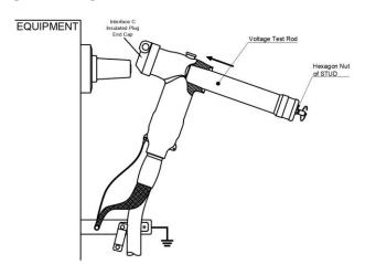
Put Interface C Insulating plug End Cap to Interface C Insulating plug. Clean and grease the test rod and front T-body interfaces. Insert the test rod into the front T-body and tighten the test rod at Hexagon Nut of stud by Hex Wrench.
