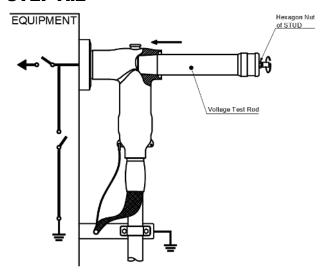
Clean and grease the test rod and front T-body interfaces. Insert the test rod into the front T-body and tighten the test rod at Hexagon Nut of stud by Hex Wrench.
