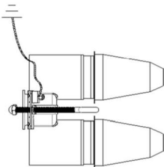
Attach #14 AWG drain wire or equivalent from the grounding lug on the feed-thru to the system ground, and leave enough slack to operate with a hotstick.
