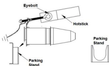
Hook the nozzle through its eyebolt, then insert it into the "Parking Stand" of the branch box or device where you want to install it, once in position, turn the eyebolt clockwise to fasten the nozzle.
