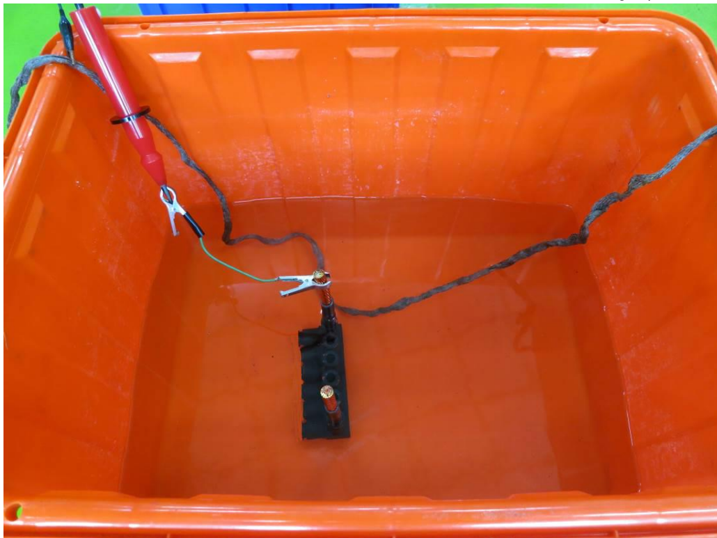
Voltage testing of the 2.2 kV 60Hz / 1min in water - II
