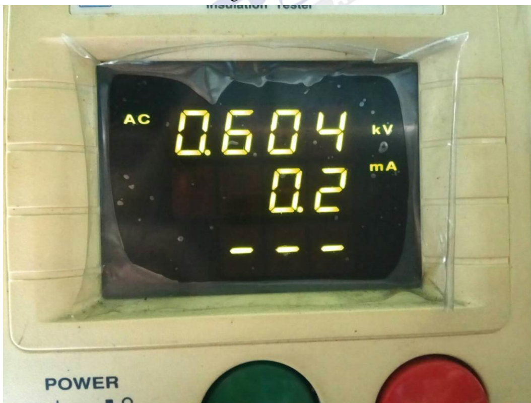
Leakage current test - II
