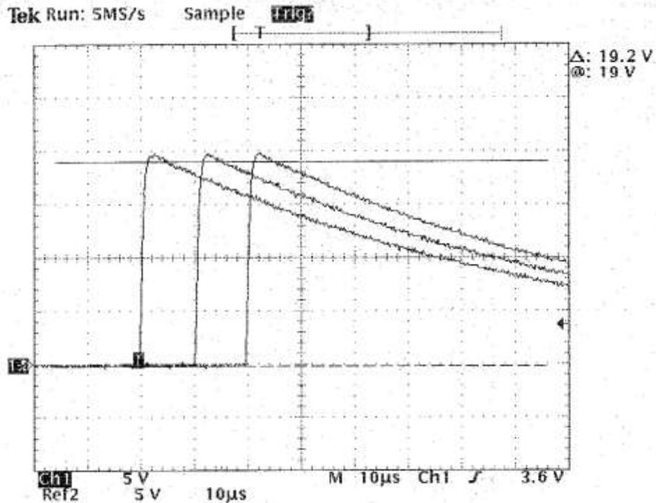
Fig 13-1 Waveform of Impulse Positive Waves after Accelerated life Sealing Test
